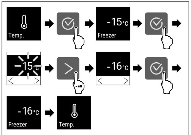
Fig. 65 Changing temperature from -15 °C to -16 °C
