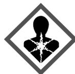
This symbol may be located on the compressor. It relates to the oil in the compressor and makes reference to the risk that: **Swallowing or inhaling can be fatal.** This advice is only relevant to recycling. There is no danger in normal operation.
