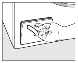
Open the drain pump access panel.
