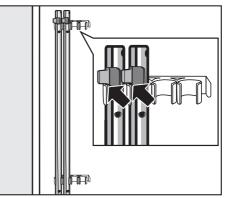
Secure the transit bars to the back of the washing machine. Make sure that the top catch is located above the holder.
