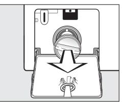
Remove the drain filter completely.
